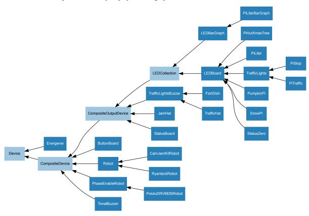
For composite devices, the following chart shows which devices are composed of which other devices:
