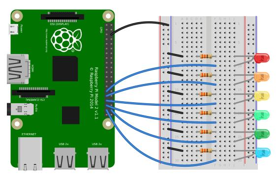
A collection of LEDs can be treated like a bar graph using LEDBarGraph (page 144):
