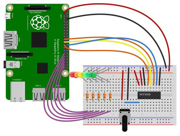
Continually print the value of a potentiometer (values between 0 and 1) connected to a MCP3008 (page 135) analog to digital converter:
