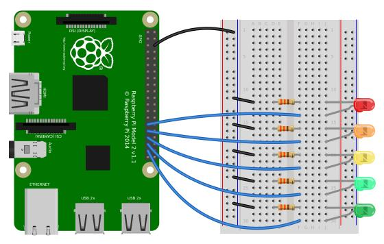
A collection of LEDs can be accessed using LEDBoard (page 141):
