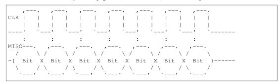
The following diagram indicates when data is read when  $clock\_polarity$  (page 203) is False<sup>913</sup>, but  $clock\_phase$  (page 203) is True<sup>914</sup>, equivalent to CPHA 1:
