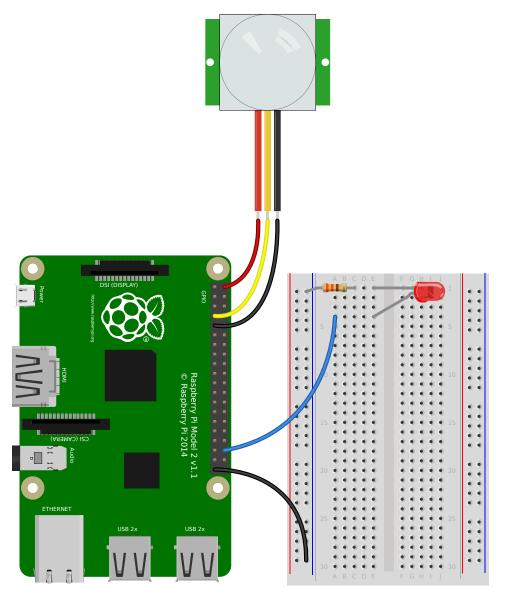
Light an  $\mbox{\it LED}$  (page 111) when a  $\mbox{\it MotionSensor}$  (page 97) detects motion:
