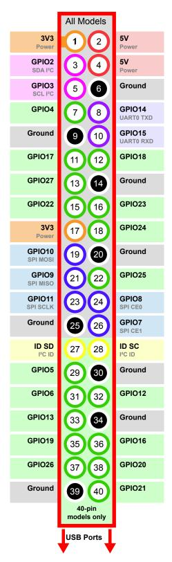
If you wish to use physical (BOARD) numbering you can specify the pin number as "BOARD11". If you are familiar with the wiringPi<sup>6</sup> pin numbers (another physical layout) you could use "WPI0" instead. Finally, you can specify pins as "header:number", e.g. "J8:11" meaning physical pin 11 on header J8 (the GPIO header on modern Pis). Hence, the following lines are all equivalent:
