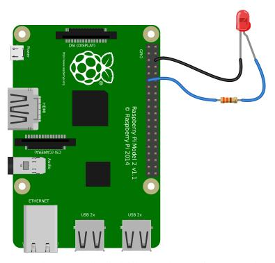
Any regular LED can have its brightness value set using PWM (pulse-width-modulation). In GPIO Zero, this can be achieved using <code>PWMLED</code> (page 113) using values between 0 and 1:
